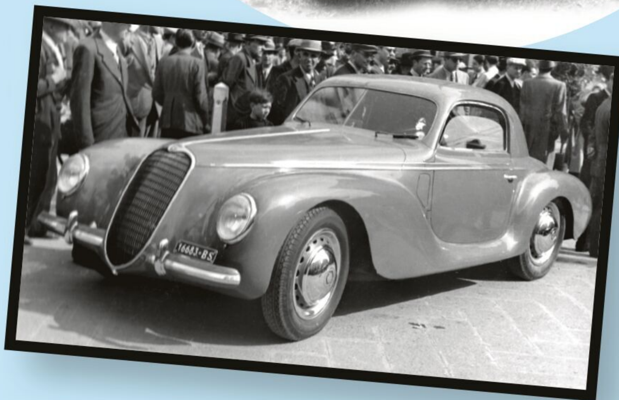
Following the success of the Mille Miglia cars, Touring moved the headlights out to the fenders. Chassis 915029
