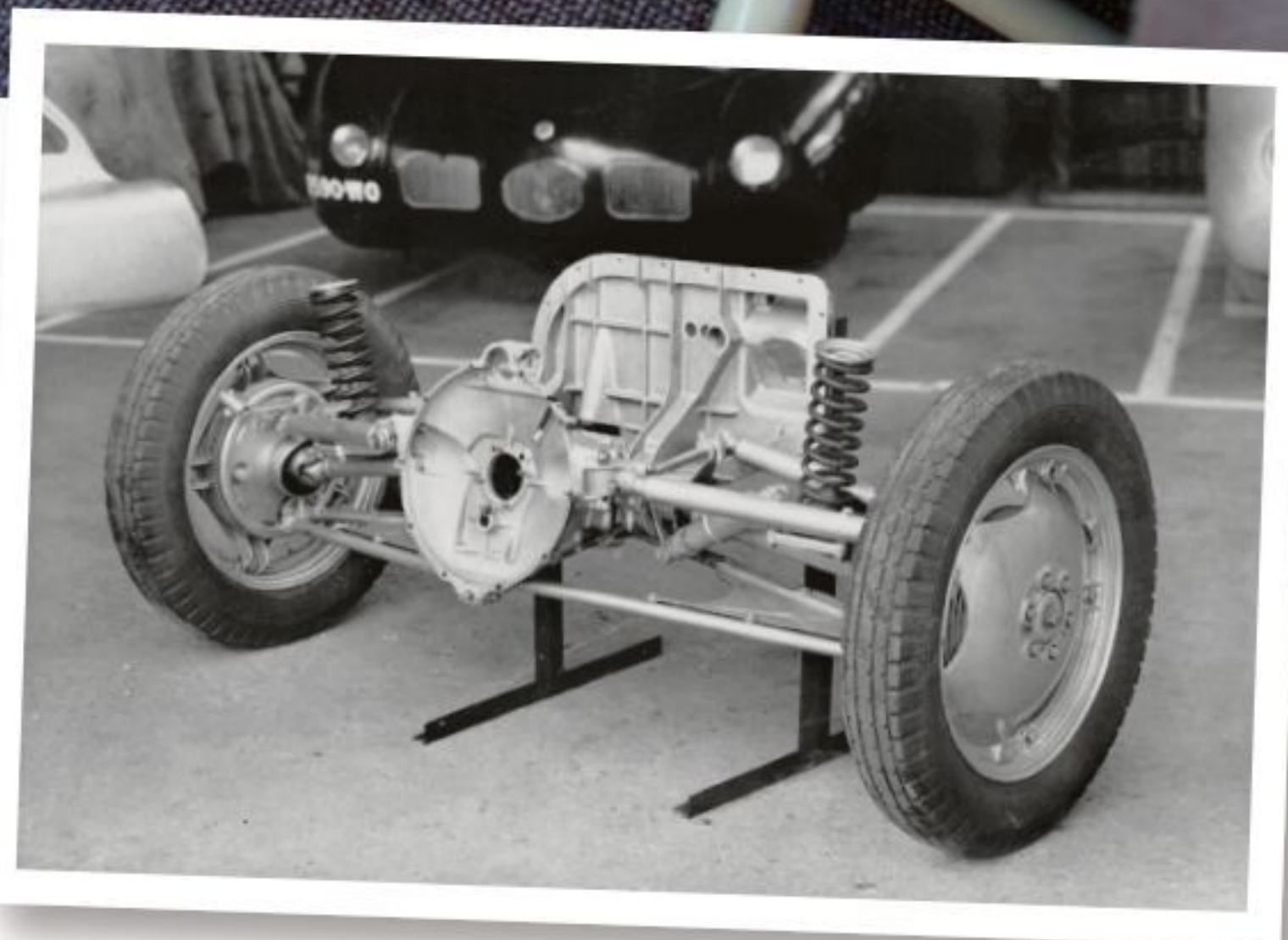
The front suspension is fully independent and uses coil springs.
