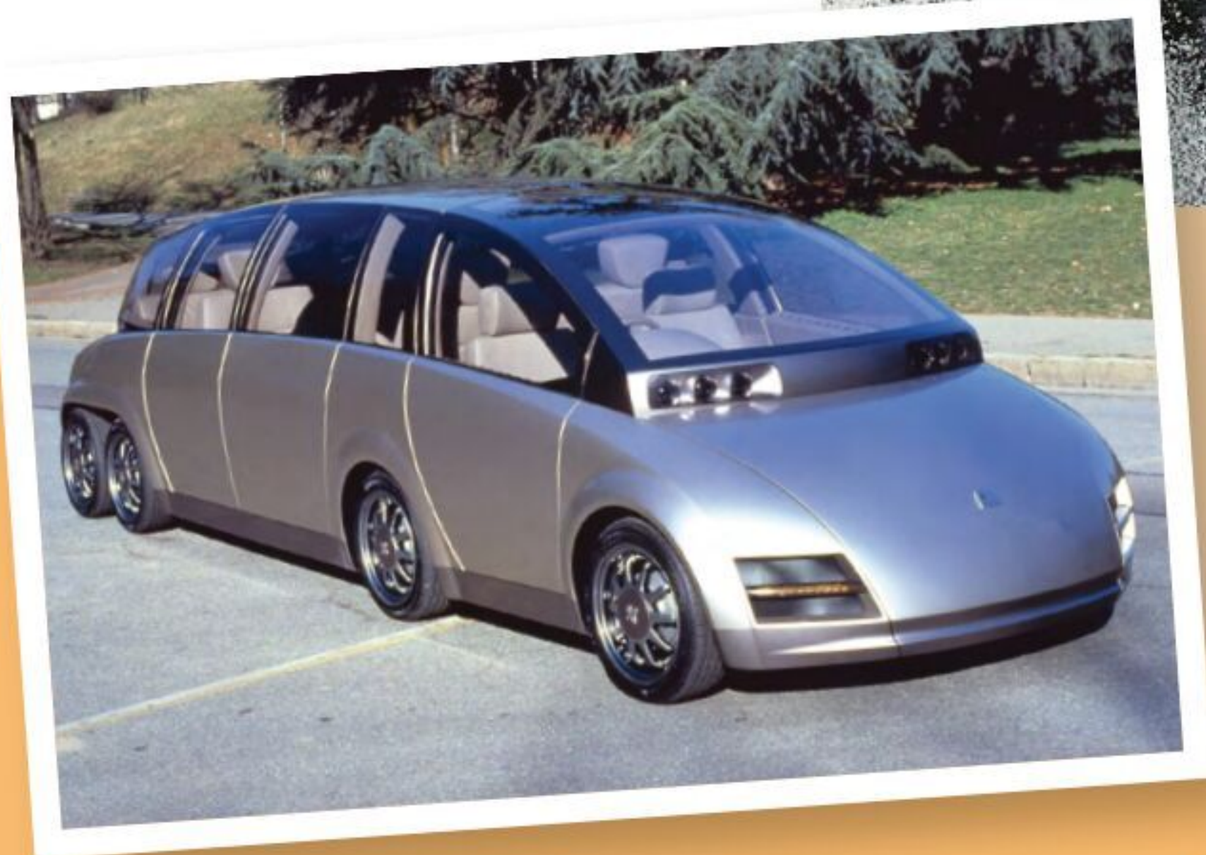
The sleek KAZ was a forward-looking eight-wheel-drive electric MPV from Japan.
