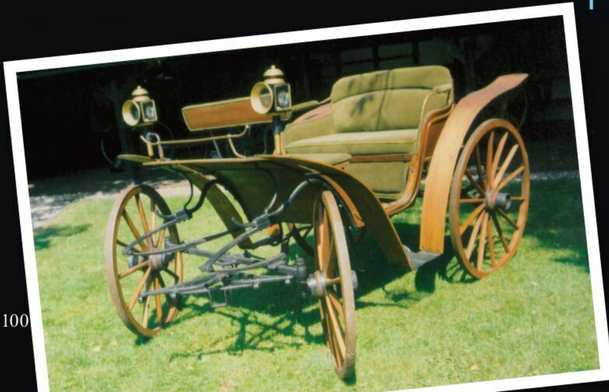
A variant on the theme: Paul Nitz was granted a patent in 1912 in Germany for his version of the trapezoid steering linkage.
