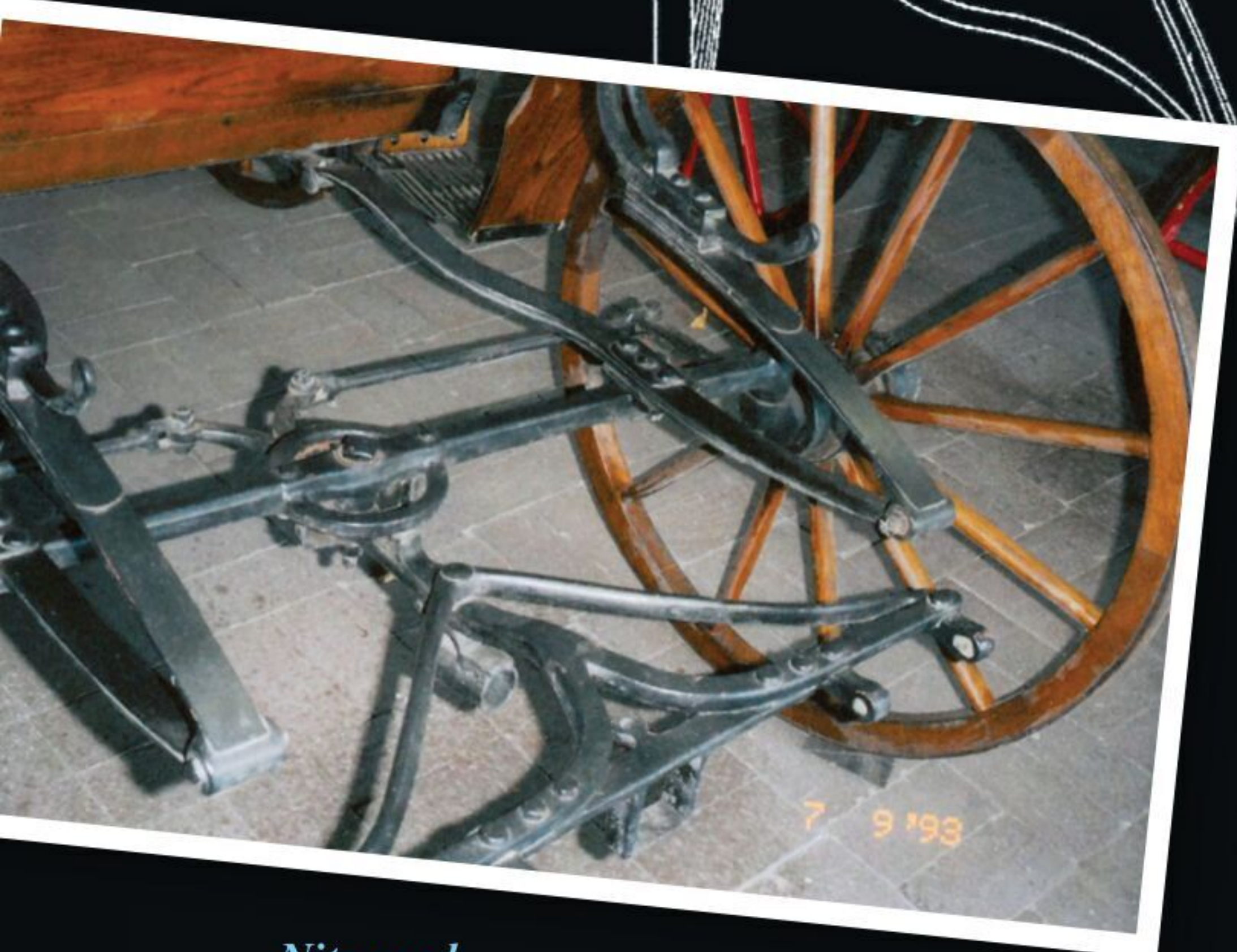
Nitz used articulated quadrilaterals.
