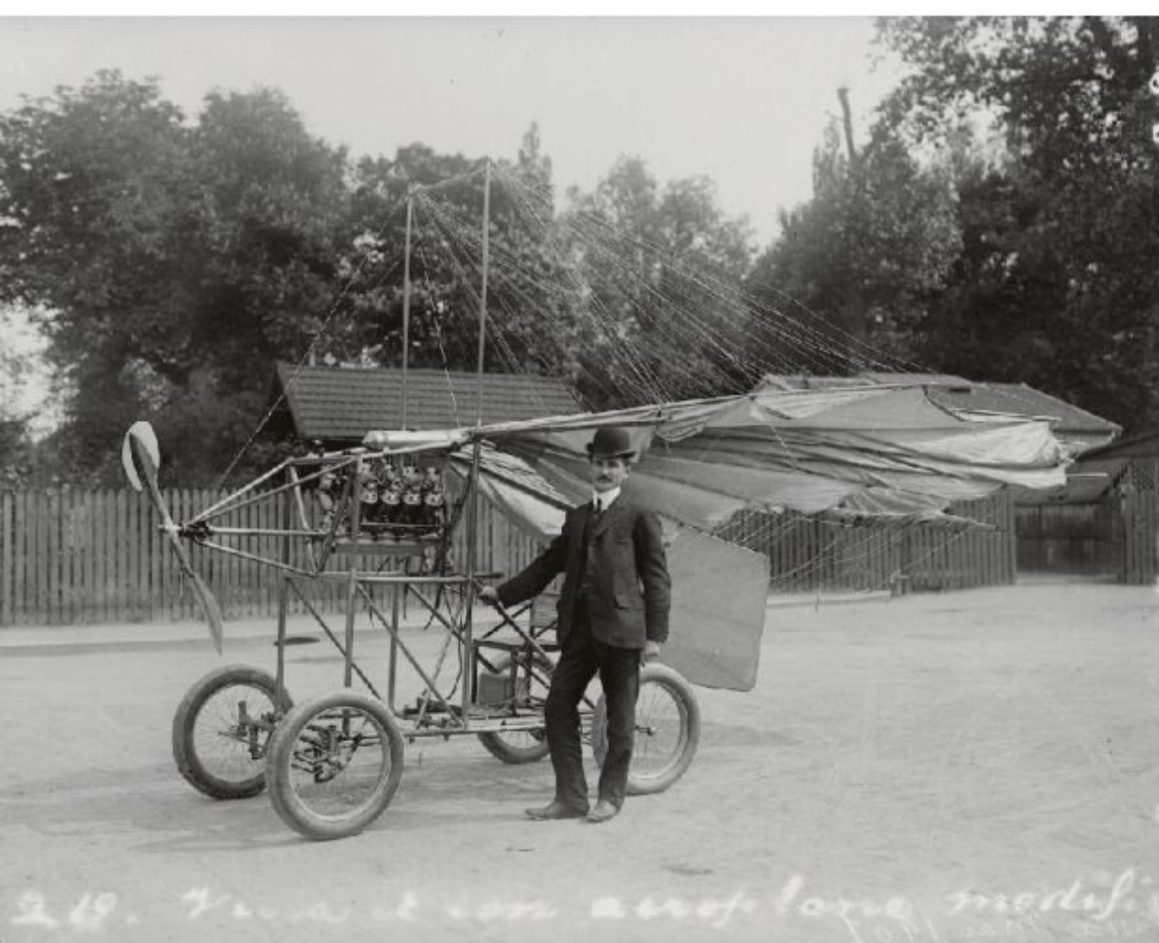
Traian Viuia's second airplane-automobile with its wings folded.
